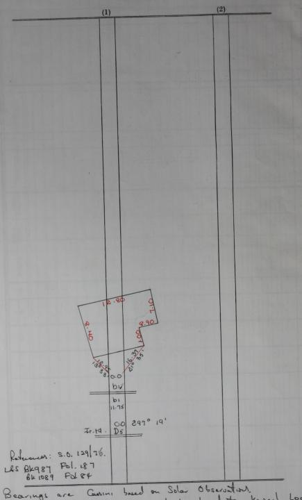
Bearings are Cousins based on Solar Observation. Surveyed in February 2002 to be leaved to knowed Lochan Distances are in METRES
