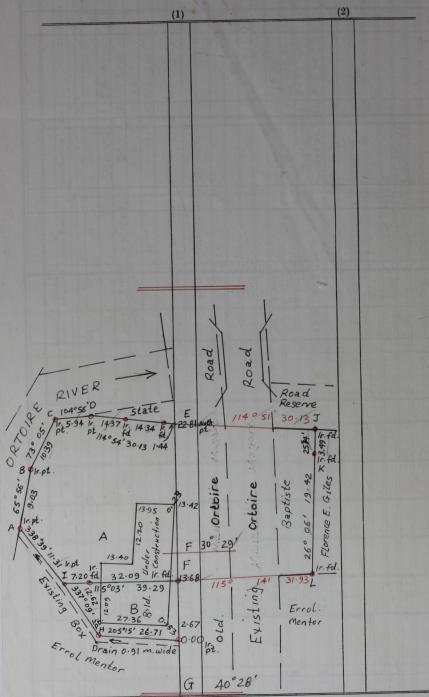
Bearings are cassini grid based on Solar Obs. Distances are in Metres
