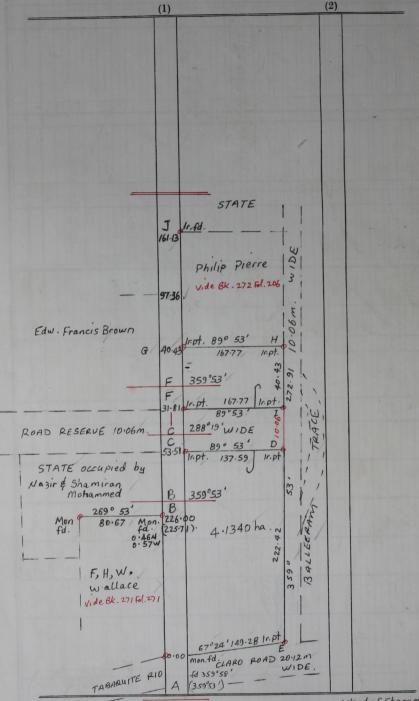
Distances are in Metres . Bearings are cassini Grid based on Solar Obs.
