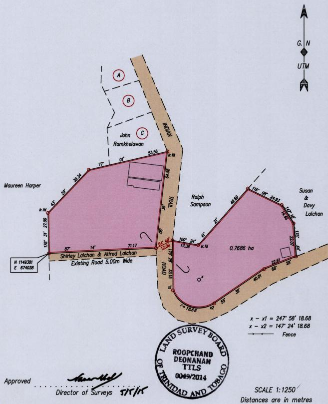
ODenotes Iron Put unless otherwise stated Bearings are UTM Grid based on Solar Observations
