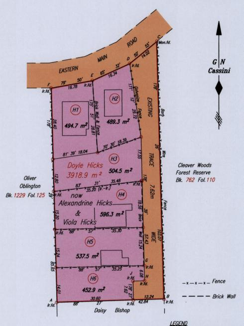
Coordinates of D (Ir.fd.): 0685866mE, 1175533mN U.T.M. 20 WGS 84 (+/- 7.00m) G.P.S. Direct Observation From To Bearing Distance
