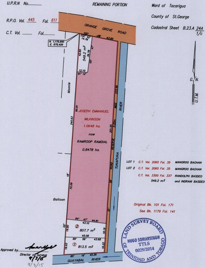
Bearings are U.T.M. Grid based on Solar Observations Note: To obtain cassini bearings add 18 minutes
