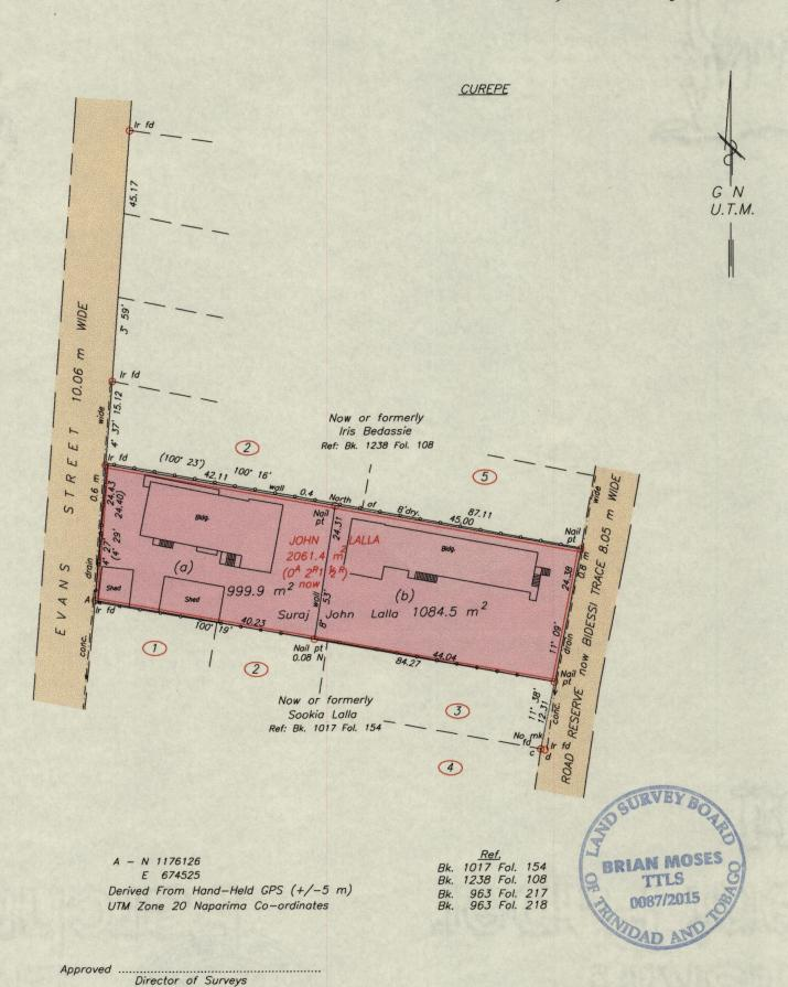
Denotes Iron put unless otherwise stated Bearings are U.TM. grid based on Solar observations SCALE 1:750
