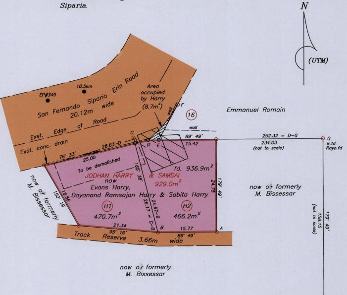
Note - UTM (Nap-Zone 20) Coordinates obtained from hand held GPS receiver + 5.00m
