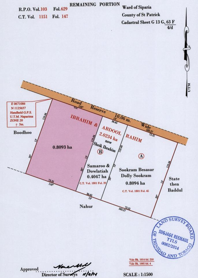
Note: Bearings are U.T.M. grid based on solar observations
