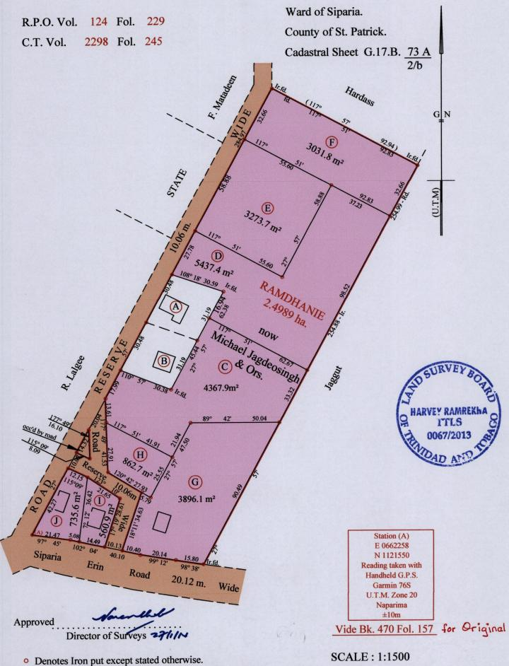
Note: Bearings are U.T.M. grid based on solar observations
