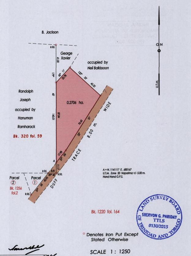
Bearings are U.T.M. Grid based on Solar Observations Distances are in Metres PLAN of a Parcel of land coloured pink in the Ward of Savana Grande Containing zero point two seven zero six hectare Surveyed by me with due authority on 17<sup>th.</sup> September 2013 for Kayshnee Seepersad Certified correct in accordance with Regulation 25 (1) of the Land Surveyors Regulations 1998.
