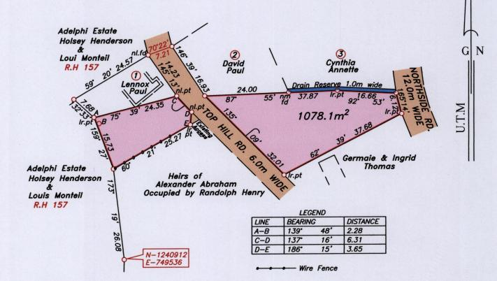
Note- UTM Zone 20 (WGS 84) Coordinates obtained from hand held GPS receiver  $^+$  5.00m
