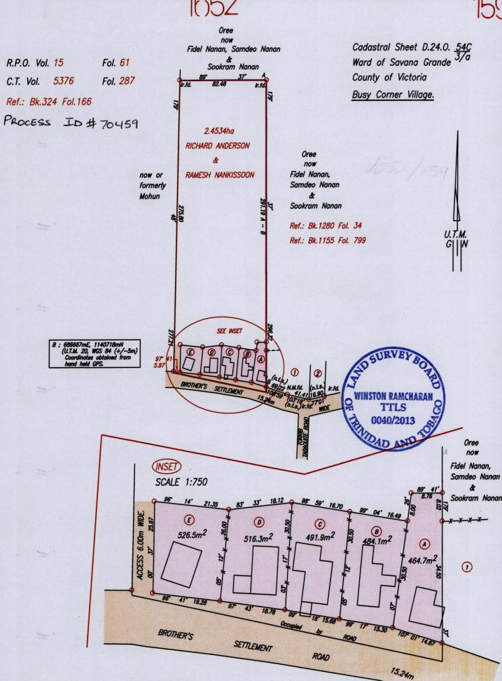
ODenotes Iron put except otherwise stated. Bearings are U.T.M. Grid based on Solar Observations.
