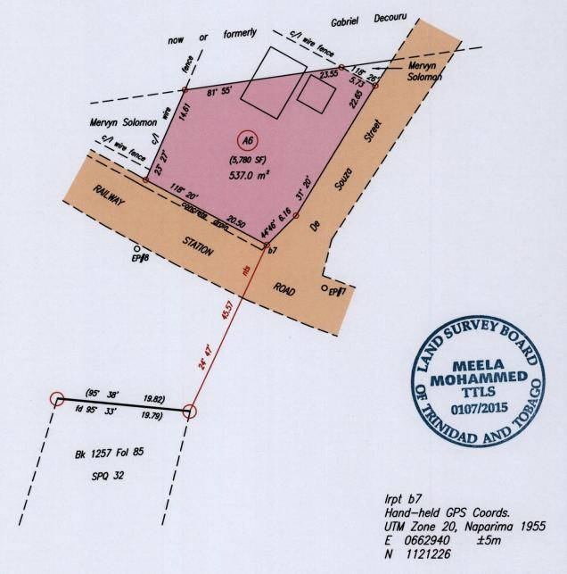
O denotes iron put except otherwise stated Bearings are Cassini Grid based on Solar Obs. Distances are in Metres SCALE 1/500
