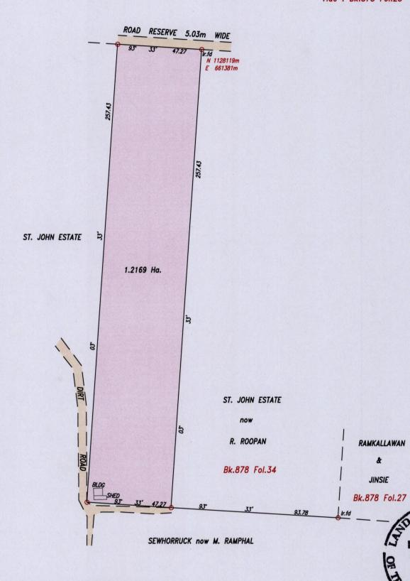
ODenotes Iron put except where otherwise stated Co-ordinates are Naparima/UTM, derived using Handheld GPS (+/-5m) Bearings are U.T.M. Grid based on Solar Observations PLAN of a Parcel of land coloured pink in the Ward of Siparia
