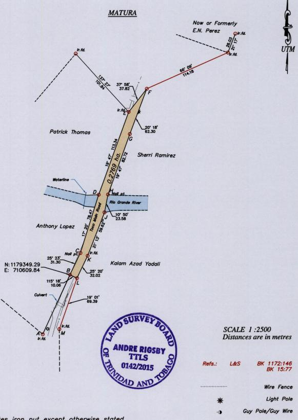
o denotes iron put except otherwise stated Co-ordinates are UTM zone 20N Naparima Datum obtained from GPS static observations Bearings are UTM grid based on Solar observations.
