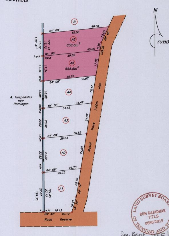
Note - UTM (Nap-Zone 20) Coordinates obtained from hand held GPS receiver + 5.00m
