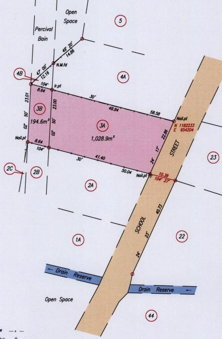
Denotes Iron found except where otherwise stated Co-ordinates are Naparima/UTM derived using handheld GPS (+/-5m)Bearings are Cassini Grid based on Solar Observations
