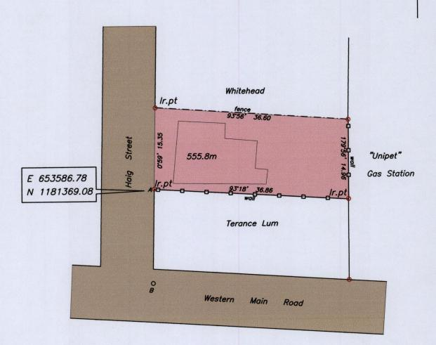
Co-ordinates are UTM zone 20N Naparima Datum +/-5m ed from Control marks Bearings are U.T.M. grid based on Control marks
