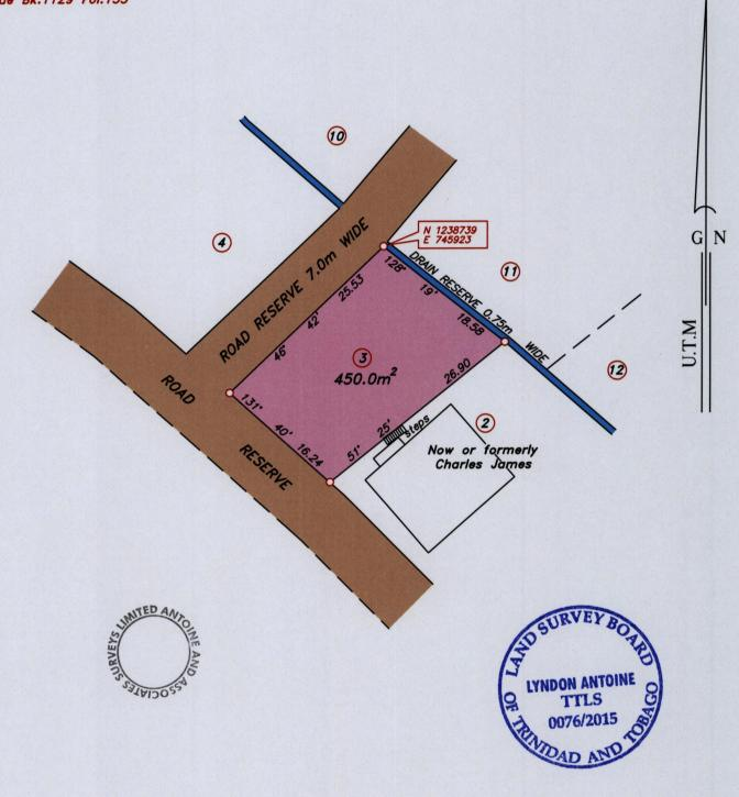
Note- UTM Zone 20 (WGS 84) Coordinates obtained from hand held GPS receiver  $\stackrel{+}{-}$  5.00m
