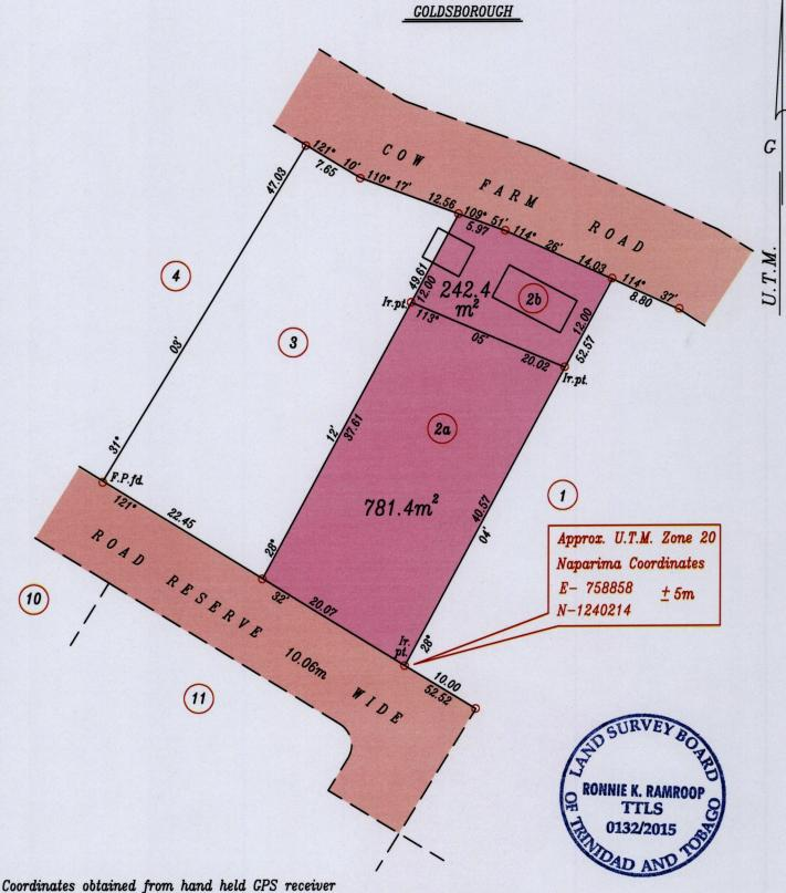
Bearings are grid based on solar observations
