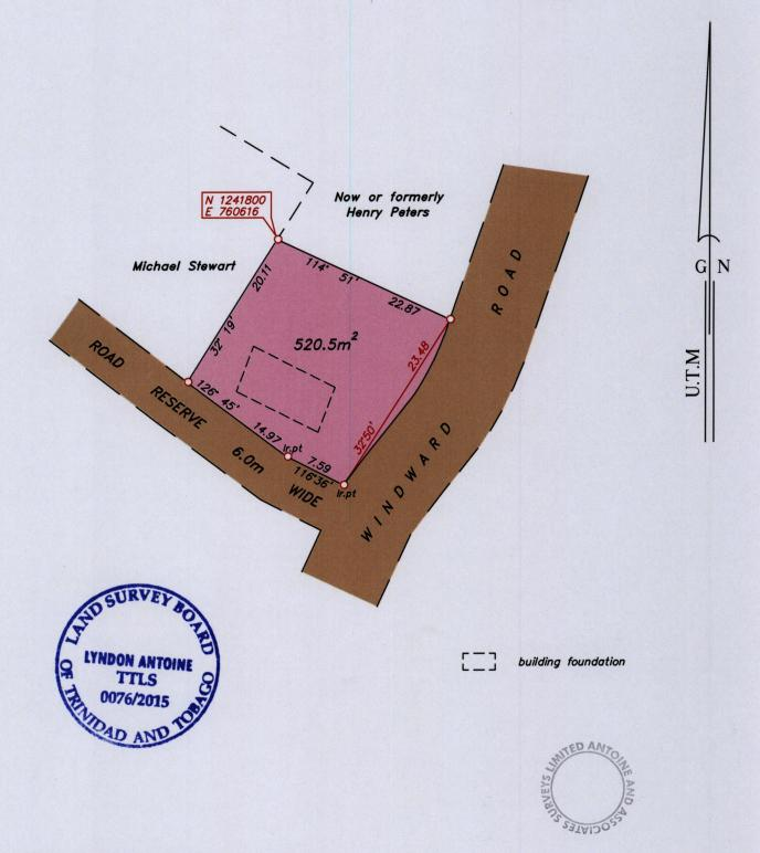
Note- UTM Zone 20 (WGS 84) Coordinates obtained from hand held GPS receiver  $^+$  5.00m
