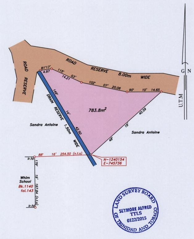
Note- UTM Zone 20 (WGS 84) Coordinates obtained from hand held GPS receiver  $\pm$  5.00m
