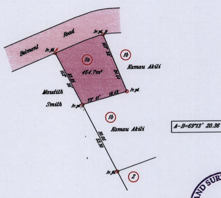
Coodinates of A (0750232mE 1240462mN) U.T.M. Naparima (-+4.00m) G.P.S. Direct observation using handheld receiver
