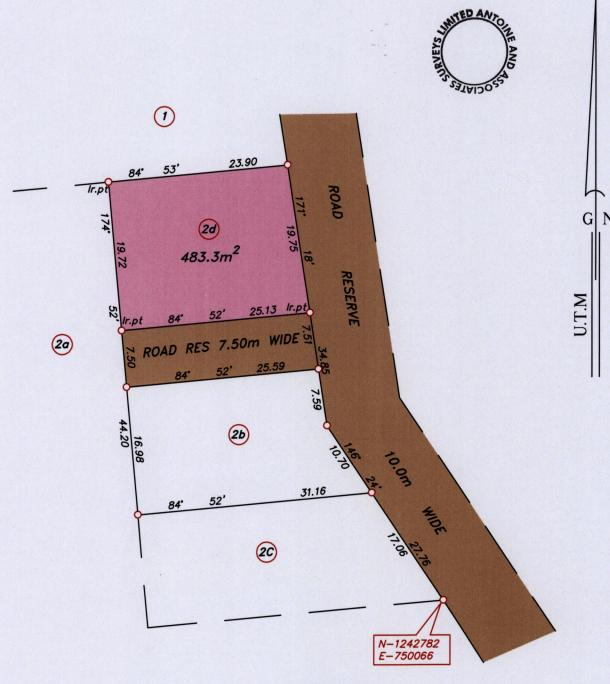
Note- UTM Zone 20 (WGS 84) Coordinates obtained from hand held GPS receiver  $\pm$  5.00m
