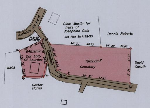
O Denotes Ir.pt. except where otherwise stated -ordinates are UTM zone 20N Naparima Datum +/-5m obtained from handheld GPS Bearings are U.T.M. grid based on Magnetic Needle
