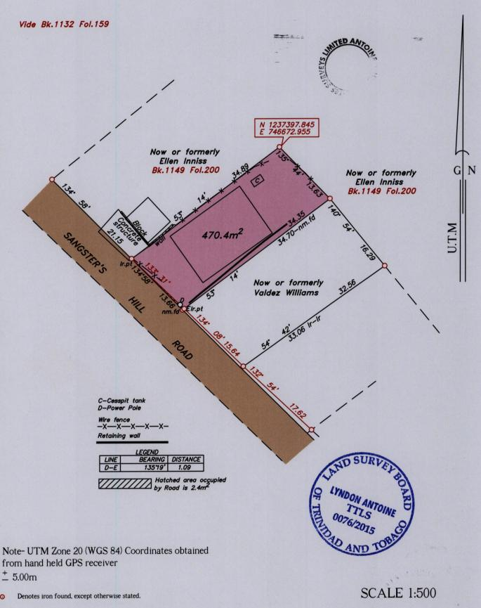
Bearings are U.T.M grid based on solar observations
