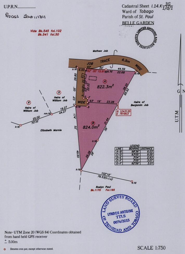
Bearings are U.T.M grid based on solar observations
