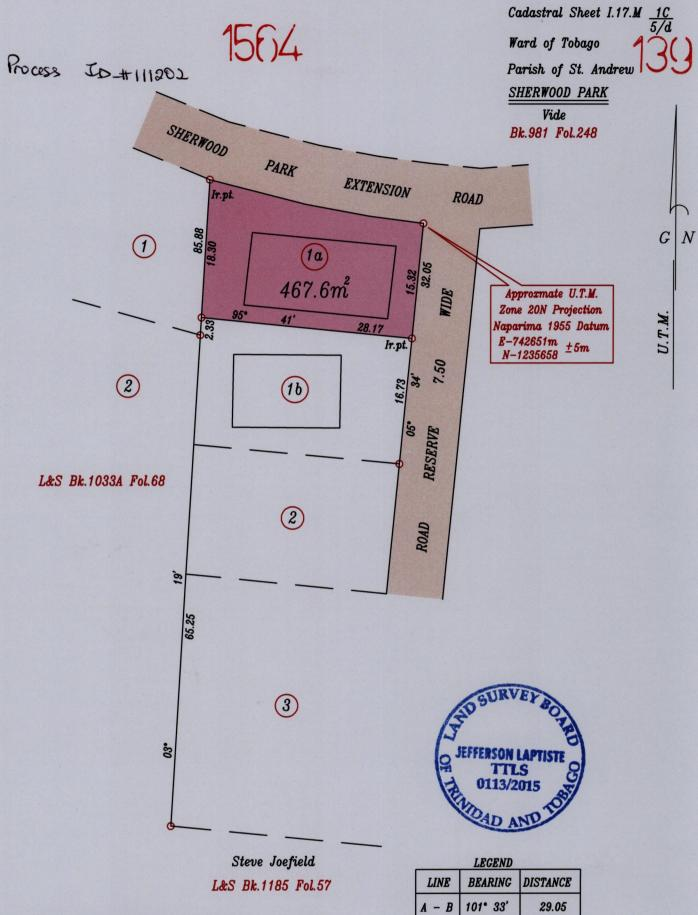
Coordinates obtained from hand held G.P.S. receiver Bearings are grid based on solar observations o denotes iron found except otherwise stated
