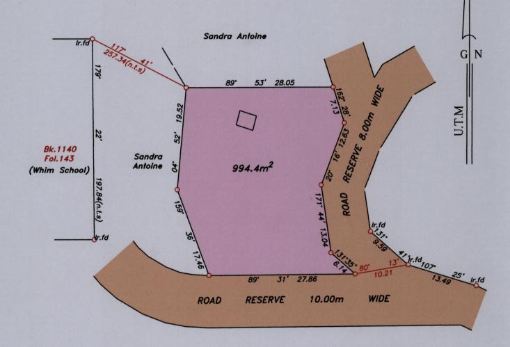
Note- UTM Zone 20 (WGS 84) Coordinates obtained from hand held GPS receiver + 5.00m
