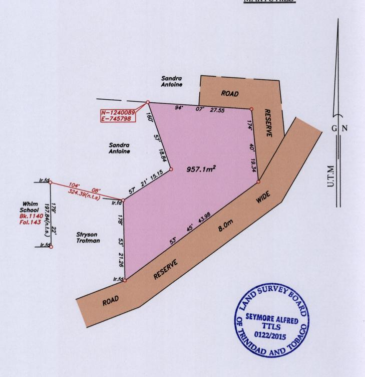
Note- UTM Zone 20 (WGS 84) Coordinates obtained from hand held GPS receiver  $\pm$  5.00m
