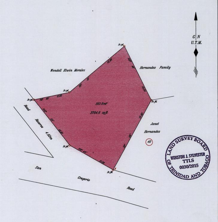
Coodinates of A (671939mE 1185474mN) U.T.M. Naparima (-+4.00m) G.P.S. Direct observation using handheld receiver
