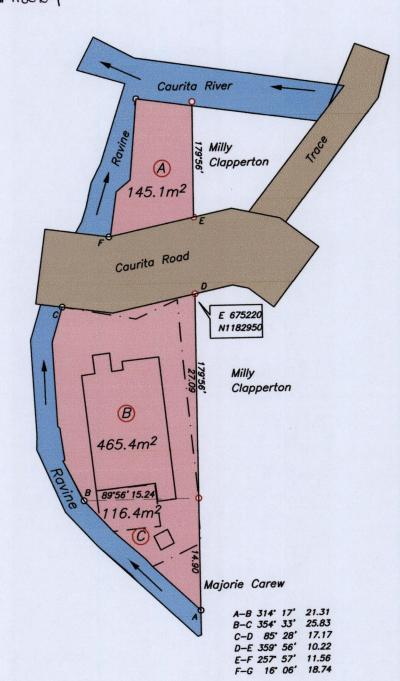
ordinates are UTM zone 20N Naparima Datum +/-5m obtained from handheld GPS Bearings are Cassini grid based on Solar Observations Note: To obtain Compass bearings add 4 minutes.
