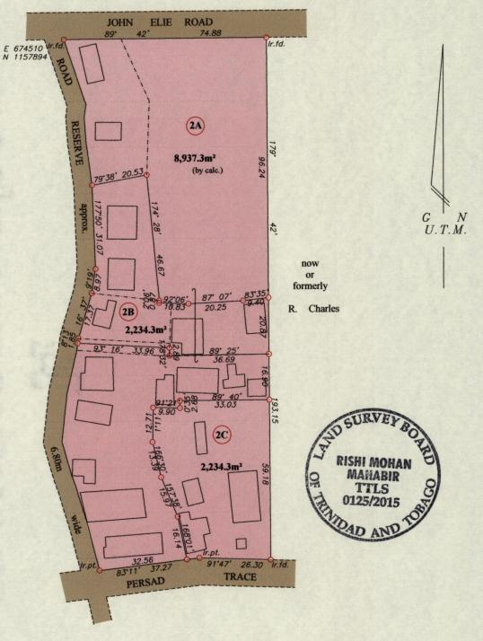
O Denotes boundary corner unless otherwise stated Co-ordinates are U.T.M. Zone 20N Naparima Datum +/-5m obtained from a handheld GPS Bearings are U.T.M. grid based on solar observations
