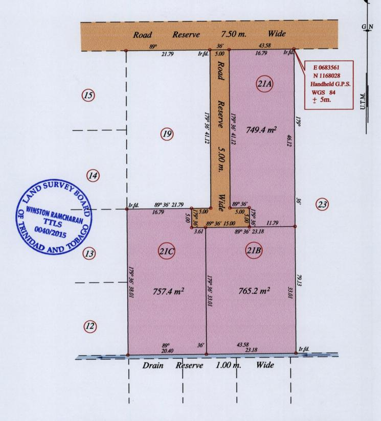
SCALE: 1:500 • Denotes Iron put except stated otherwise. Distances are in metres Note: Bearings are U.T.M. grid based on solar observations PLAN of 3 Parcels of land coloured pink in the Ward of Cunupia Containing together two thousand two hundred and seventy two point zero square metres Surveyed by me, with due authority, in May 2015 for Morris Elisha Bashay Certified correct in accordance with Regulation 25 (1) of the Land Surveyors Regulations 1998.
