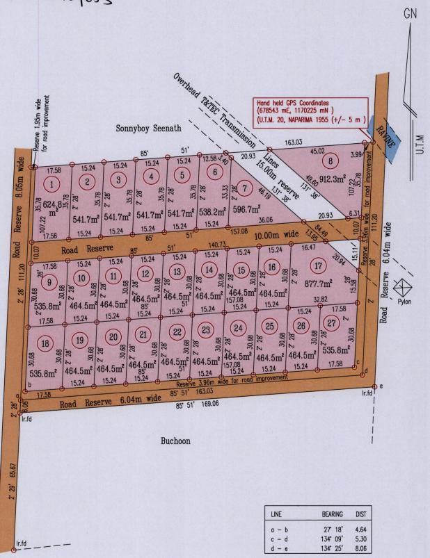
Bearings are U.T.M Grid based on Solar Obs.
