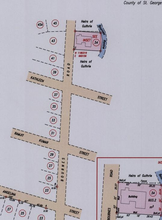
ODenotes Iron put except where otherwise stated Bearings are U.T.M. Grid based on Solar Observations Co-ordinates are Naparima/UTM, derived using Handheld GPS (+/-5m) PLAN of a Parcel of land coloured pink in the City of Port-of-Spain Containing six hundred and three point two square metres Surveyed by me, with due authority, in April 2015 for Nkomo Kamau Certified Correct in accordance with Regulation 25 (1) of the Land Surveyors' Regulations 1998,
