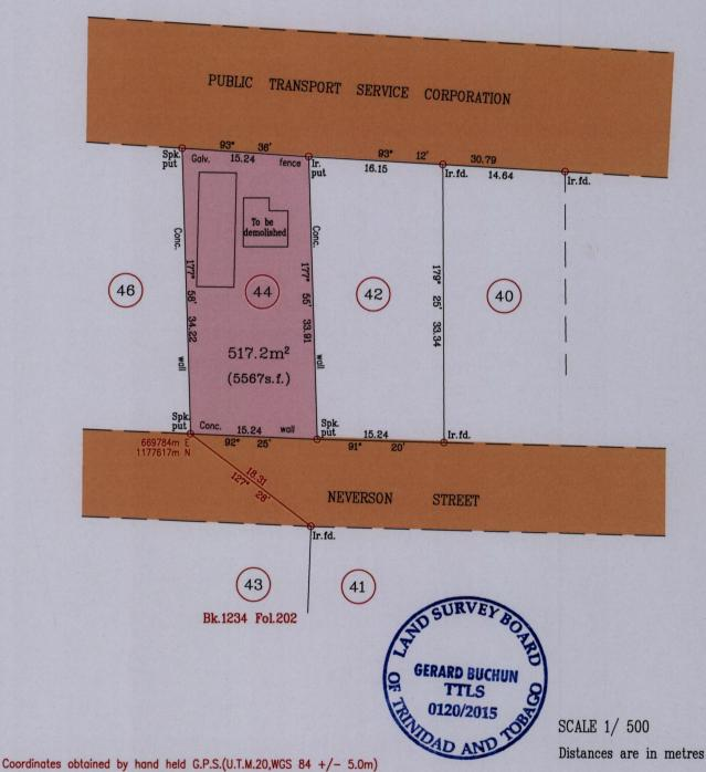
Bearings are U.T.M. Grid based on Solar Observations.
