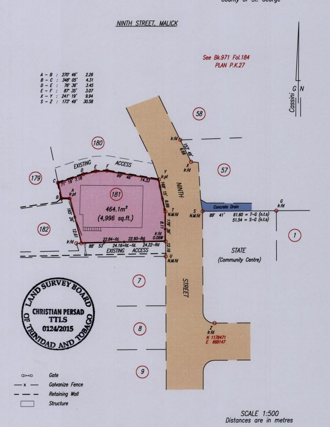
O Denotes Nail Put except where stated otherwise Bearings are Cassini Grid based on Solar Observations Co-ordinates are Naparima 1955/UTM, derived using Handheld GPS (+/-3m)
