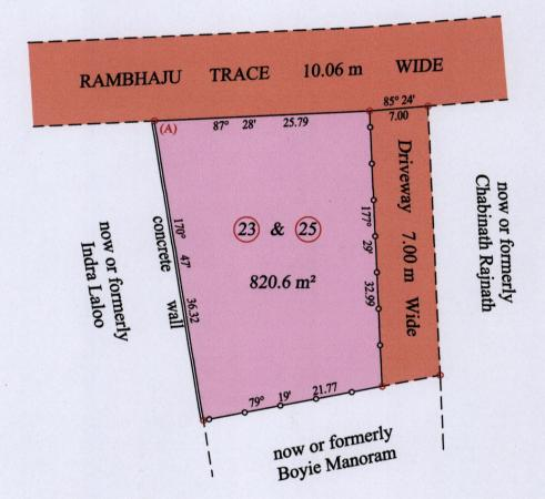
At Station (A) E 0669909 N 1175714 Reading taken with Handheld G.P.S. U.T.M. Zone 20 Naparima + 5 m.
