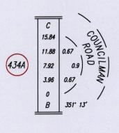
O Denotes Iron Put except where stated otherwise Bearings are UTM Grid based on Solar Observations Co-ordinates are Naparima 1955/UTM, derived using Handheld GPS (+/-3m) SCALE 1:500 Distances are in metres
