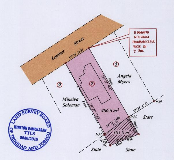
SCALE: 1:500 Denotes Iron put except stated otherwise. Distances are in metres Note: Bearings are U.T.M. grid based on solar observations PLAN of 2 Parcel of land coloured pink in the Ward of St. Anns Containing together five hundred and ninety one point six square metres Surveyed by me, with due authority, in December 2014 at the request of Yvonne Welch Certified correct in accordance with Regulation 25 (1) of the Land Surveyors Regulations 1998.
