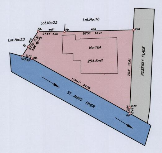
O denotes Ir.pt except otherwise stated Co-ordinates are UTM zone 20N Naparima Datum +/-5m Obtained from handheld GPS Bearings are UTM grid based on Solar Observations Note: To obtain compass bearings add 18 minutes.
