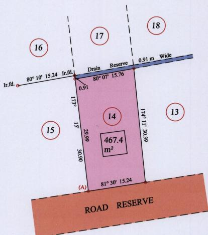
At Station (A) E 0682112 N 1136243 Reading taken with Handheld G.P.S. U.T.M. Zone 20 WGS84
