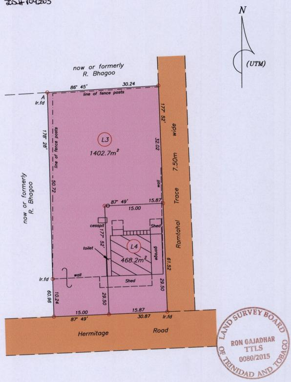
Note - UTM (Nap-Zone 20) Coordinates obtained from hand held GPS receiver + 5.00m
