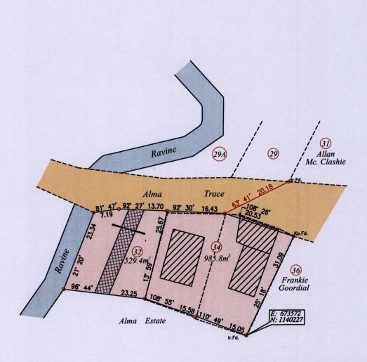
Southern boundary line adjusted as per request by current owner, Pooran Ramroop which supersedes southern boundary line as defined in previous survey plan Bk:1172 Fol 217
