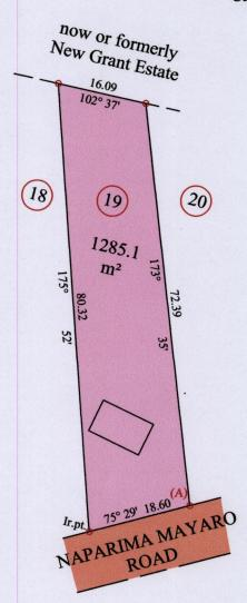
At Station (A) E 0682705 N 1136393 Reading taken with Handheld G.P.S. U.T.M. Zone 20 Naparima + 5 m.
