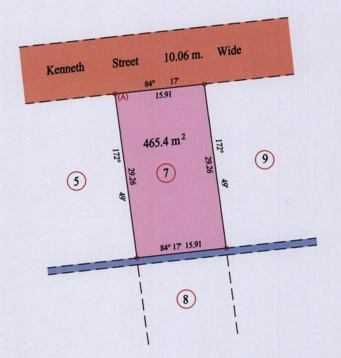
At Station (A) E 0644475 N 1124966 Reading taken with Handheld G.P.S. U.T.M. Zone 20 Naparima + 5 m.
