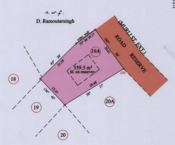
At Station (A) E 0665276 N 1132928 Reading taken with Handheld G.P.S. U.T.M. Zone 20 Naparima + 5 m.
