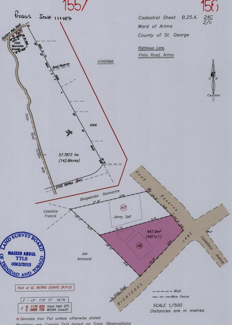
Bearings are Cassini Grid based on Solar Observations PLAN of a Parcel of land coloured pink in the Ward of Arima Containing four four seven point nine square metres Surveyed by me, with due authority, in June 2015 for Augustine Lambkin Certified Correct In accordance with Regulation 25 (1) of the Land Surveyors' Regulations 1998,
